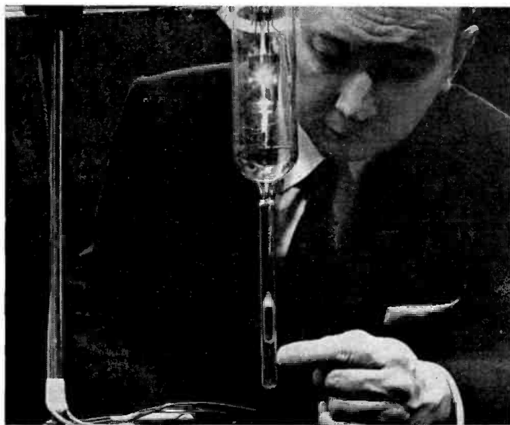
Power Sources. Exotic power sources are under research. They make use of the latest advances in chemistry and physics. This experimental thermionic tube, which converts heat directly into electricity, is a possible new source for producing electric power in the future.
